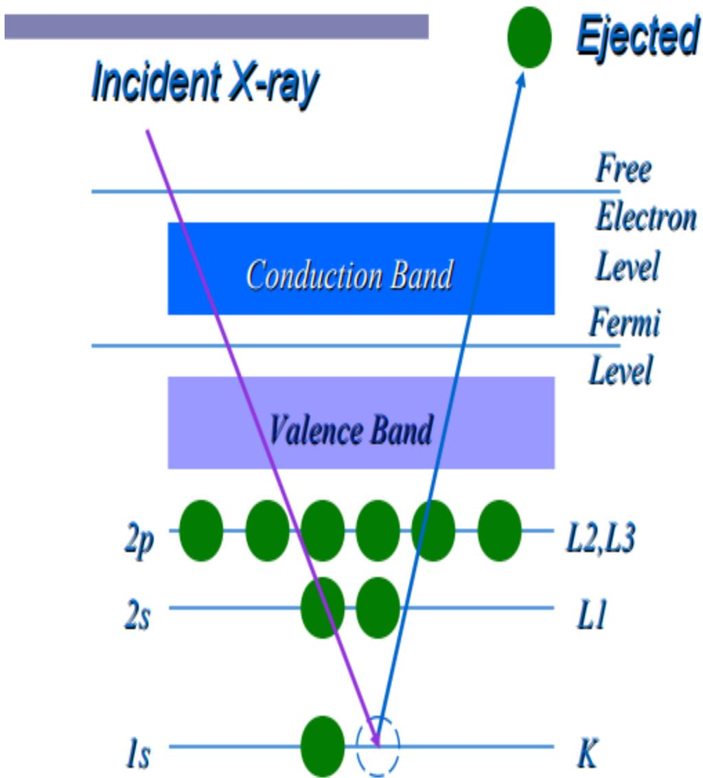
XPS spectral lines are identified by the shell from which the electron was ejected (1s, 2s, 2p, etc.). The ejected photoelectron has kinetic energy:
